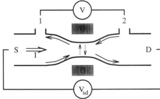
FIG. 1. Schematic of quantum Hall bar with gated constriction ( $G$ ) separating source from drain. Of interest are nonequilibrium fluctuations in the current,  $I$ , and voltage,  $V$ , in the presence of an applied source-to-drain voltage,  $V_{sd}$ .
