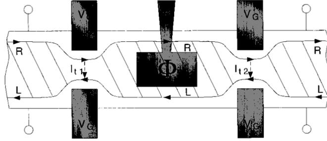
Figure 3: Two-point contact quantum Hall interferometer
